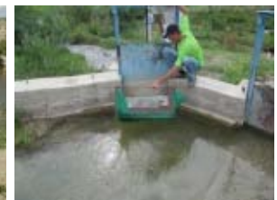
Figure 4. Measurement of water discharge
