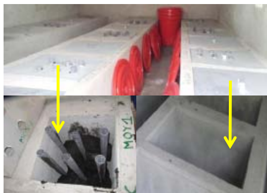
Photo 1. Different experimental storage vaults of human excreta
