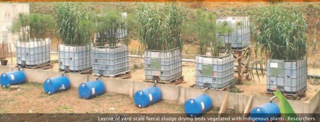
tested the ability of antelope grass and papyrus to serve as supporting material for faecal sludge treatment in Cameroon. Photo: Ives Kengne
