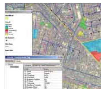
Figure 4: The main element of the NakInfo interface is a digital map with a high-resolution satellite image in the background, onto which the user can display one or several layers of spatial information. A legend allows for the easier understanding of the symbology and a query tool provides tabular information on selected map elements.
