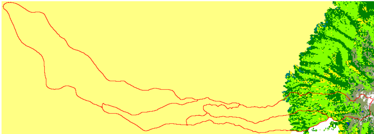
Fig. 7.13: Land use under the scenario lcsc05. The ochre areas to the left are Gb (>50% bare grassland). The areas above 3200 m a.s.l. remain unaffected. Catchment boundaries A3 – A6 are shown in red.
