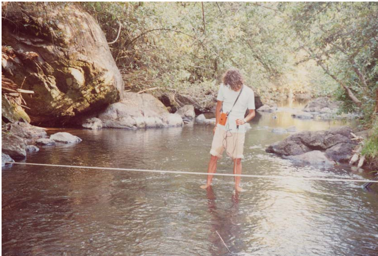
Fig 4.6: Current meter gauging on Burguret River (picture by J. Aeschbacher)
