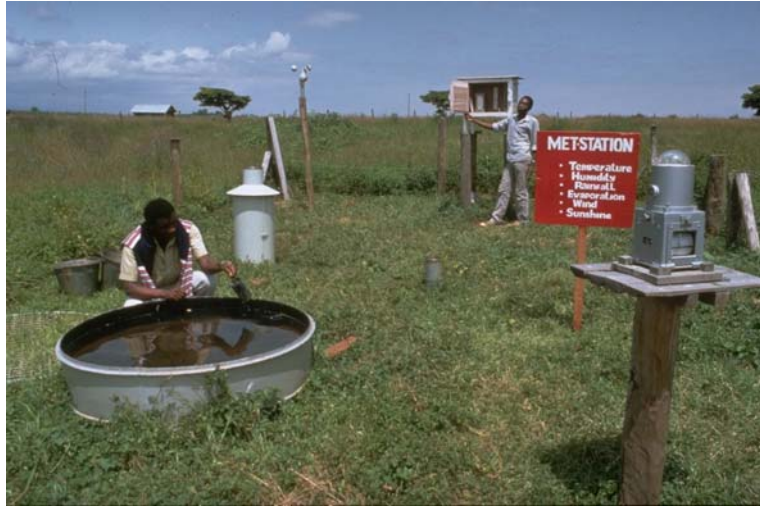
Fig. 4.2: An NRM 3 Met Station with an evaporation pan (left foreground) and a rain gauge behind it (picture by Hanspeter Liniger).
